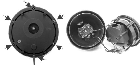
4. To detach the battery connection wire, press the clip on the connector and then pull it out. NOTE: Wrap the connector immediately with insulating tape in order to avoid short circuit caused by contact of both wire terminals.
