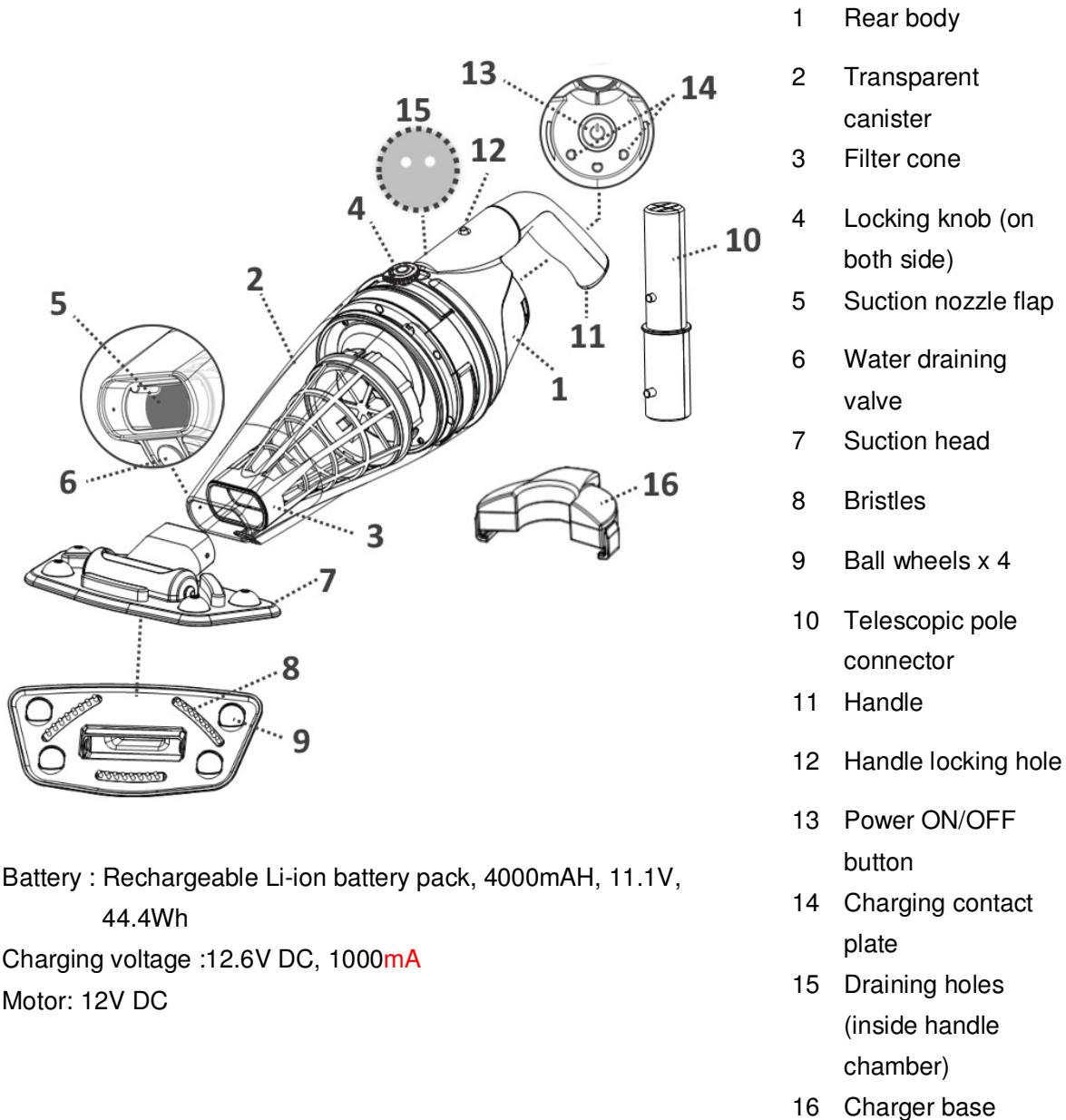
**Battery :** Rechargeable Li-ion battery pack, 4000mAH, 11.1V, 44.4Wh
