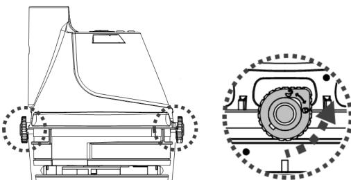
2. Place the rear body (upside down - power on/off button face up) on a flat surface. Align and slide the hook of the charging base onto the side notch at the bottom of the rear body until it stops. Make sure their contact plates are properly in contact. Plug the female jack of the external adaptor into the charging port at the end of the charging base.
