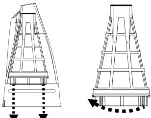
4. Rinse the transparent case and clean out the debris inside the filter cone. It is recommended to clean the filter cone's net with splashing water. If brushing is deemed
